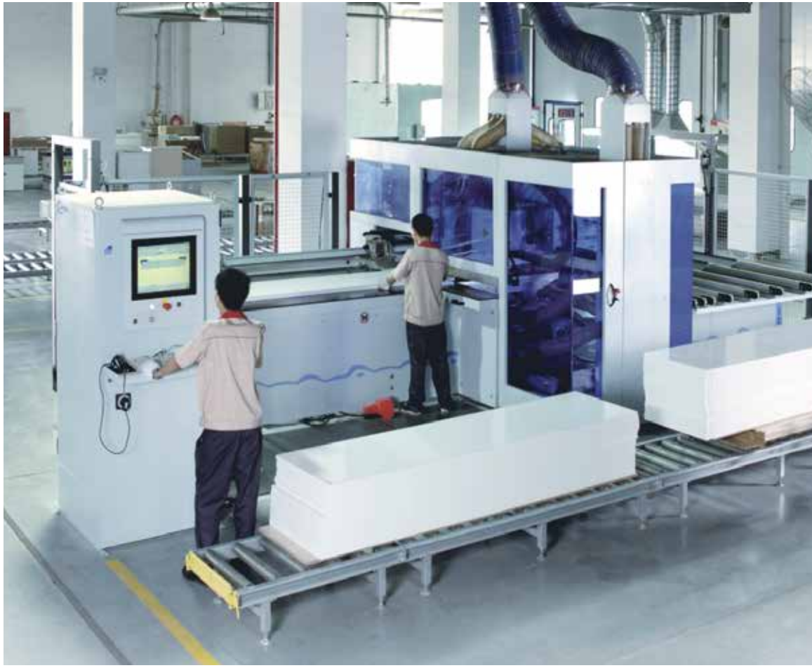
German Homag drilling machine computer controlled
